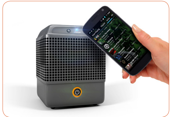
Figure 7. One-tap from an NFC-enabled device simplifies Bluetooth pairing
