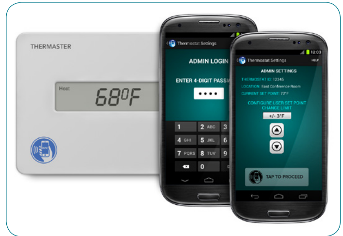
Figure 3. Controlled access to thermostat settings
