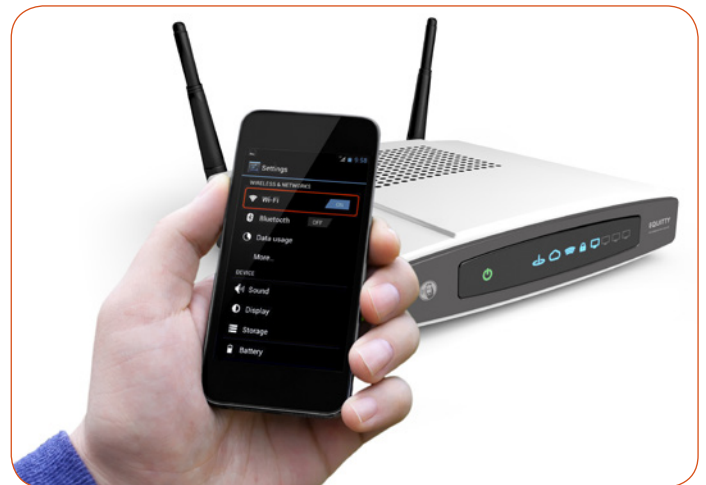
Figure 8. An NFC-enabled device passes network credentials to WiFi routers
