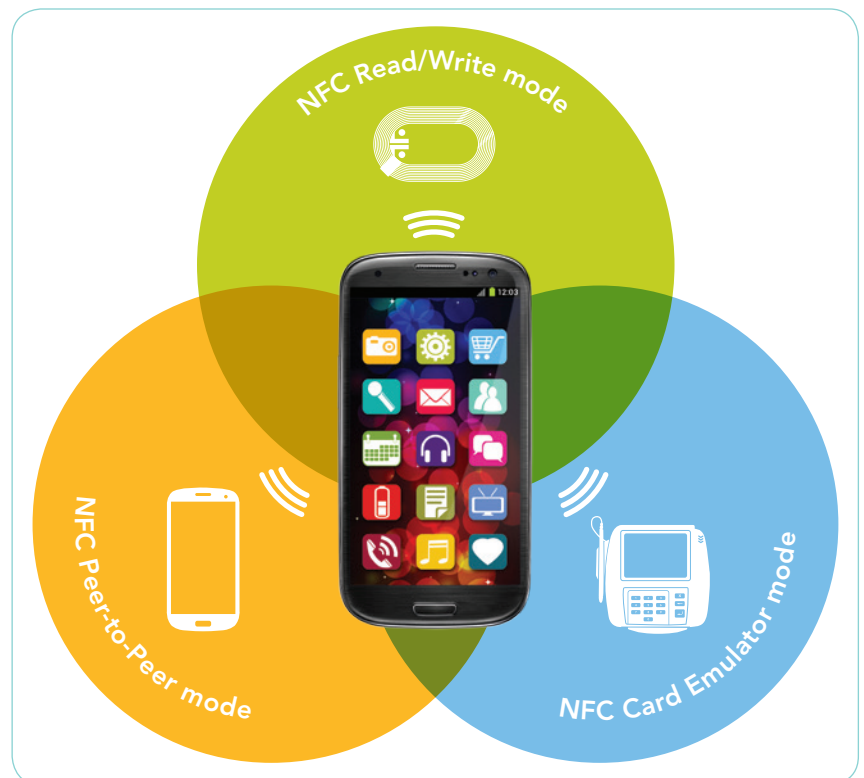
Figure 1. The three modes of NFC communication
