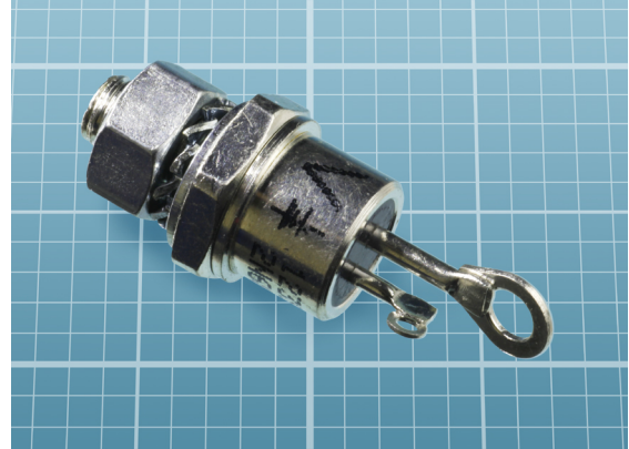
Figure 1-5. Stud-packaged SCR rated for 50V repetitive off-state voltage, no greater than 25A RMS.
