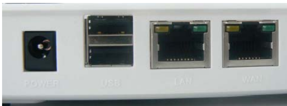
Figure 3. Ethernet and USB Ports on MPC8308-NSG
