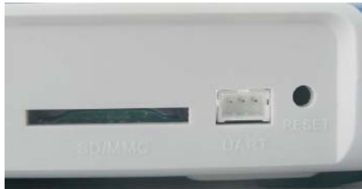
Figure 4. UART Port and SD/MMC Slot on MPC8308-NSG
