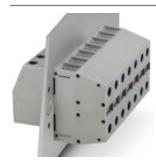
Panel feed-through terminal block, connection method: Screw connection, Screw connection, number of positions: 1, load current: 125 A, cross section: 6 mm² - 35 mm², AWG 10 - 2, connection direction of the conductor to plug-in direction: 90 °, width: 15.1 mm, color: gray
