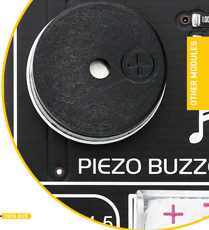
Figure 29: Piezo buzzer with the schematic
