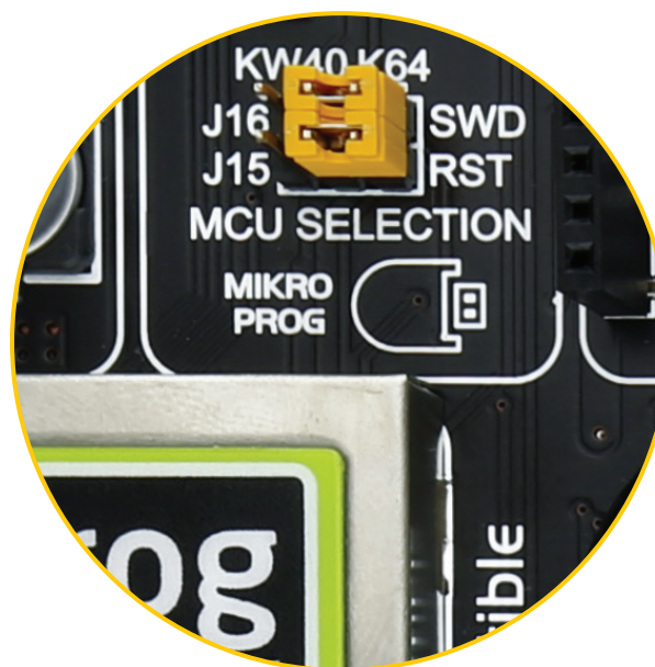
Figure 12: Target MCU selection jumpers
