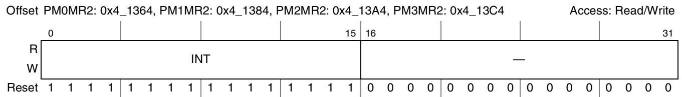
Figure 10-27. Performance Monitor n Mask Registers 2 (PM n MR2)
