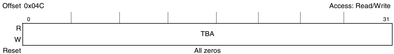
Figure 21-10. Trace Buffer Address Register (TBAR)
