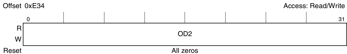
Figure 18-34. PCI Express Error Capture Register 3 (PEX_ERR_CAP_R3) Internal Source, Outbound Transaction
