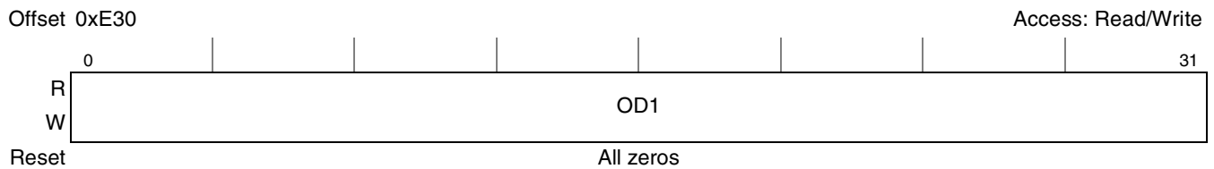
Figure 18-32. PCI Express Error Capture Register 2 (PEX_ERR_CAP_R2) Internal Source, Outbound Transaction
