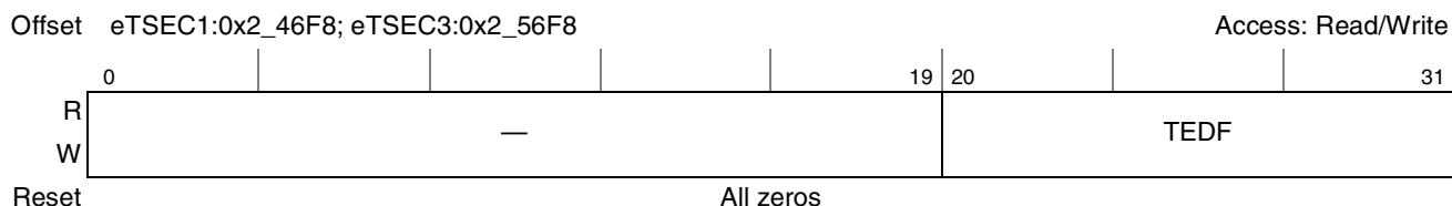
Figure 15-82. Transmit Excessive Deferral Packet Counter Register Definition
