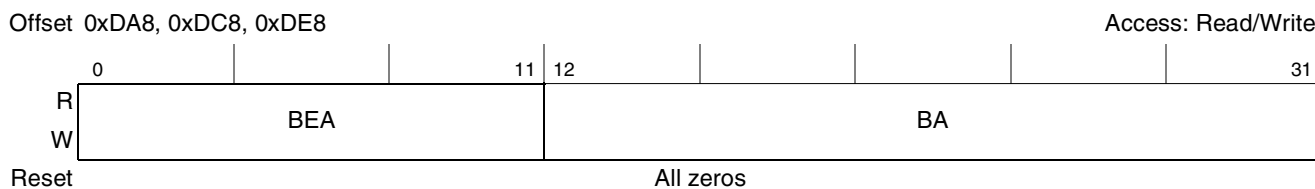
Figure 17-12. PCI Inbound Window Base Address Registers
