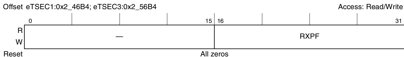
Figure 15-65. Receive Pause Frame Packet Counter Register Definition
