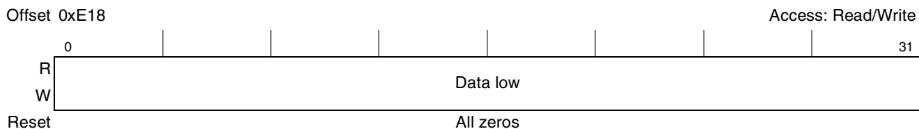
Figure 17-21. PCI Error Data Low Capture Register (ERR_DL)
