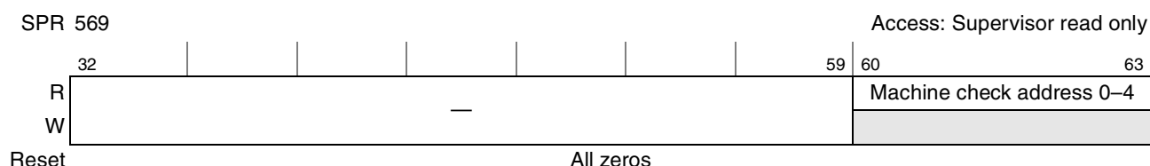
Figure 6-26. Machine Check Address Register Upper (MCARU)
