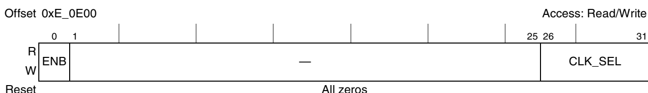
Figure 19-23. Clock Out Control Register (CLKOCR)
