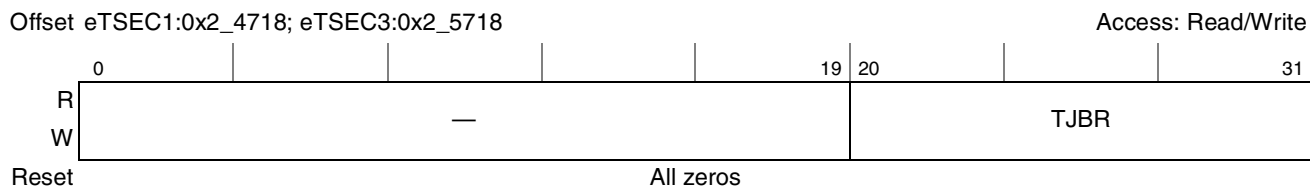
Figure 15-89. Transmit Jabber Frame Counter Register Definition
