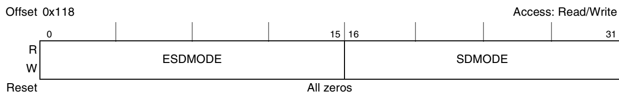
Figure 9-10. DDR SDRAM Mode Configuration Register (DDR_SDRAM_MODE)
