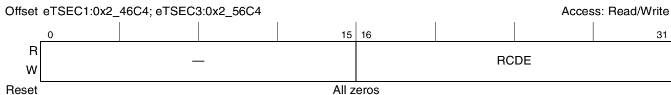
Figure 15-69. Receive Code Error Counter Register Definition
