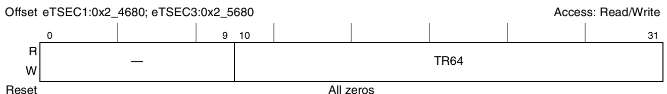
Figure 15-52. Transmit and Receive 64-Byte Frame Register Definition
