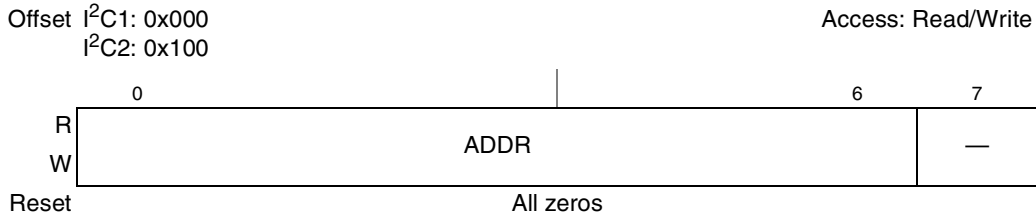
Figure 11-2. I 2 C Address Register (I2CADR)
