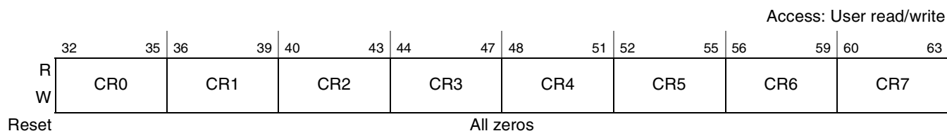
Figure 6-3. Condition Register (CR)
