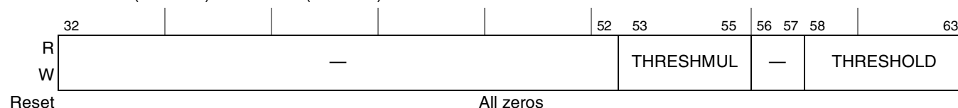
Figure 6-60. Local Control B Registers (PMLCb0–PMLCb3)/User Local Control B Registers (UPMLCb0–UPMLCb3)
