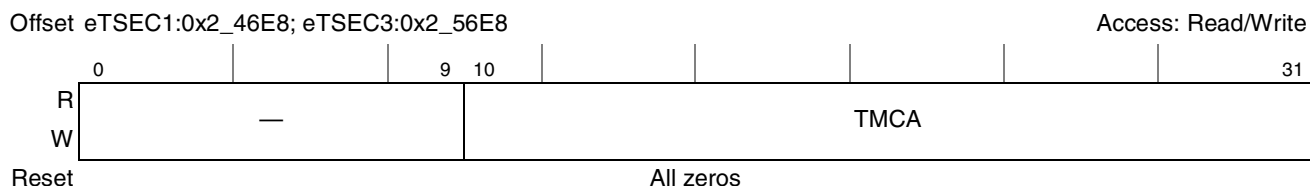
Figure 15-78. Transmit Multicast Packet Counter Register Definition
