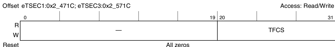
Figure 15-90. Transmit FCS Error Counter Register Definition
