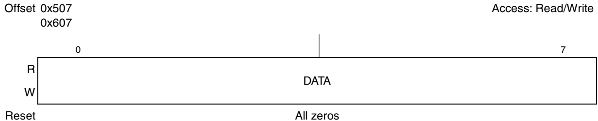
Figure 13-13. Scratch Register (USCR)
