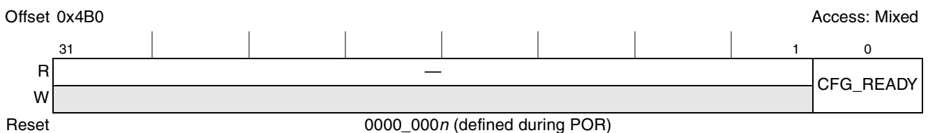
Figure 18-119. PCI Express Configuration Ready Register (PEX_CFG_READY)
